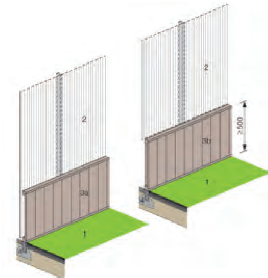
Figure 11 – perimeter fencing with containment panels used when the synthetic turf surface is laid up to the perimeter of the field
